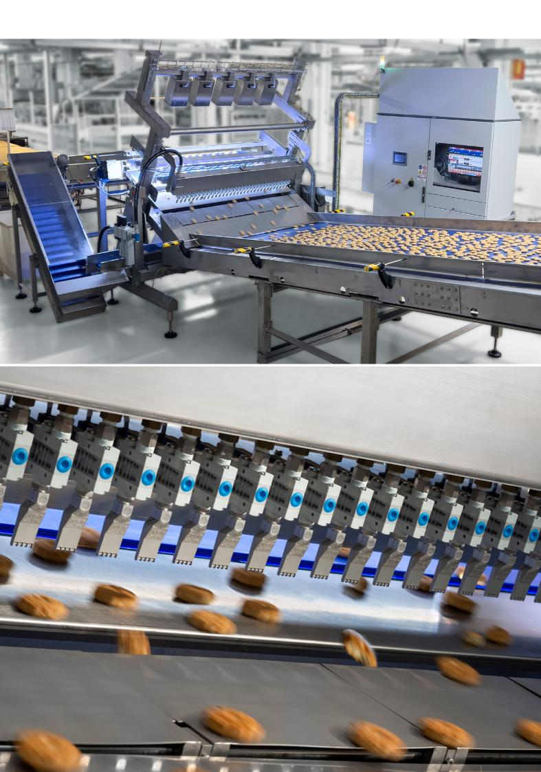
SENSURE STARGATE ML-C is an innovative vision system that, thanks to the use of SENSURE SYNAPSE technology, allows you to perform the quality control of highly variable products and automatically reject noncompliant ones. SENSURE STARGATE ML-C also guarantees continuous monitoring of the process with data collection and analysis, providing a real-time display and dedicated reporting.
