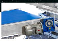
Customized **conveyors for products** handling at the entrance and exit of SENSURE STARGATE ML-C.
