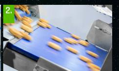
Easily interchangeable polizene plate for products sliding (low friction system and compliant with regulations required in the food industry).
