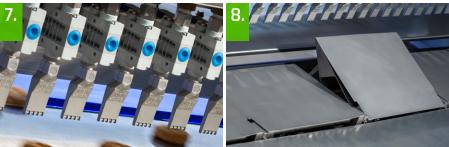
Air nozzles for the rejection of the single non-compliant product.
